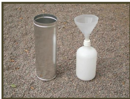
**Figure 1. Bulk Collector**
