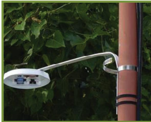
**Figure 2. Samplers mounted under rain shield**
